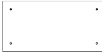
1b. Panel Mechanically fixed to exposed hammered concrete wall
