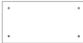
2. Panel Mechanically fixed to smooth wall or panel (concrete, plasterboard, timber panel, timber door or metal sheet)
